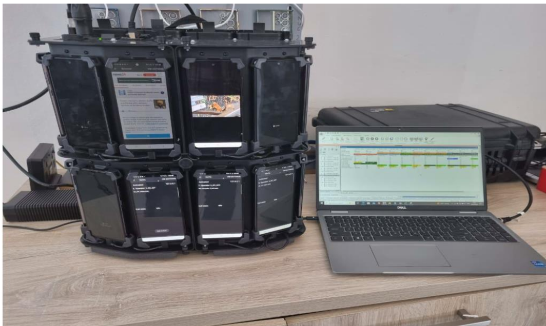
Figure 2. Drive Test System hardware configuration
